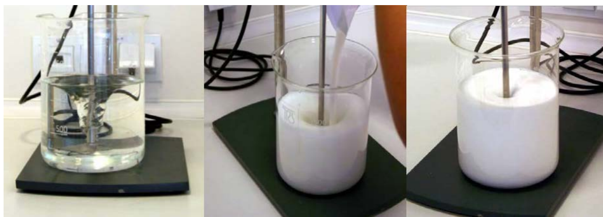
Figure 1. a: Propeller stirrer properly positioned in mixing vessel. b: Addition of Aquarius™ film coating system powder to the water. c: Mixing for 60 minutes
